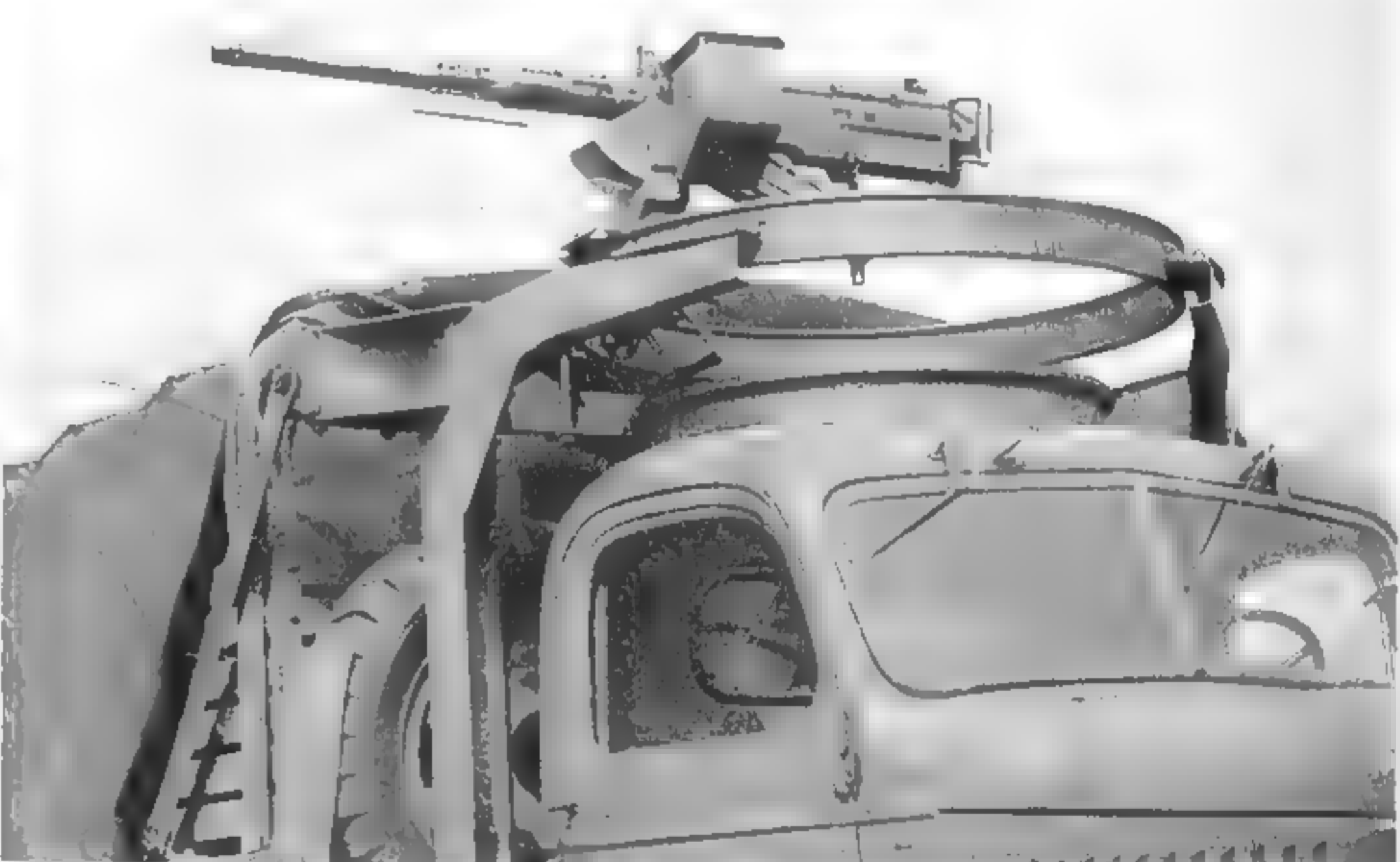
The closed-cab CCKW-352 utilized the M37 mount to attach its anti-aircraft weapon. Unlike the M32, only a small reinforcement extends to the rear of the front of the bed. Variations of this mount were used on short-wheelbase trucks with wooden beds, as well on long-wheelbase CCKW tanker trucks. (U.S. Army photo)
